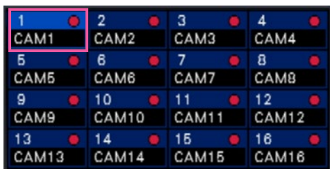
Camera No. box in the control screen
