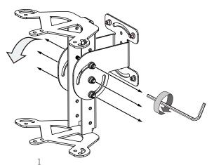
3. Secure the illuminators to the brackets using 4 included hex socket screws. If preferred, you can turn the illuminators to be facing outwards to avoid over-lapping the IR light coverage areas.
