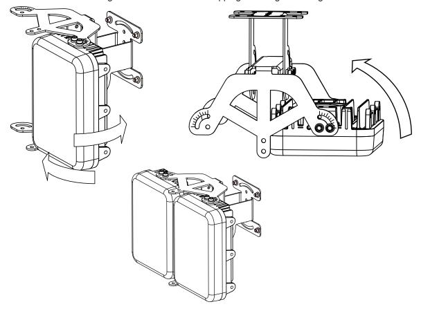
Type 2 Installation: 3 Illuminators Using the CMA-B06 Extension Bracket
