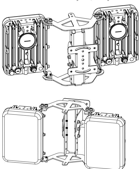
4. Install another illuminator to the center. Adjust the pan and tilt angles if preferred.
