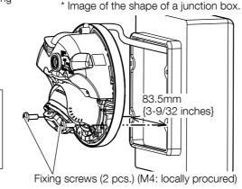
After the camera is secured, connect power to the system. (power from a PoE hub, etc.)
