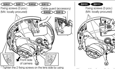
the slotted holes on the front side of the camera.
