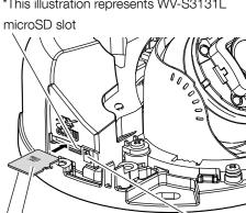
microSD memory card (the Symbol of side with printing facing up) the microSD
