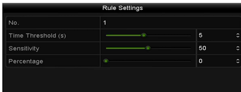
Figure 10-7 Set Intrusion Crossing Detection Rules
