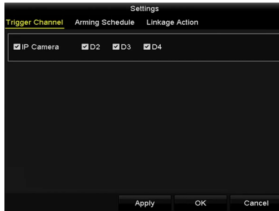
Figure 5-19 Set Trigger Camera of VCA Alarm
