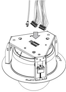
9. Use a #2 Phillips screwdriver to loosen (turning clockwise) the clamping plates, and then insert the recessed-mount bracket through the pre-drilled hole in the ceiling.
