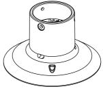
7. Turn the assembly over and place it carefully on the foam blocks that came with the shipping package to prevent damage to the dome cover. Secure the anti-tamper screws from the openings on the bracket using the included T25 stardriver.
