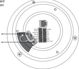
5. Fasten the black M4 machine screws to secure the interface section of the camera to the recessed-mount bracket.
