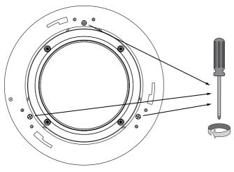
10. Use a #2 Phillips screwdriver to move the clamping plates down so that the ceiling/ board is caught between the clamps and the flange on the other side of the ceiling.
