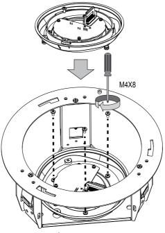
6. Attach the camera body to the interface section by aligning the indicator mark on the camera with that on the interface section. Turn the camera counter-clockwise until the indicator mark is aligned with the "C" mark.
