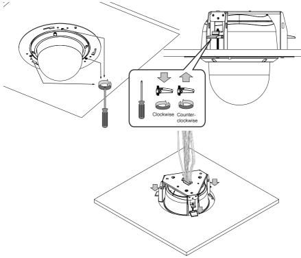
11. Align and attach cover ring to the bracket by turning it counter-clockwise.
