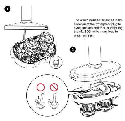
Attach the AM-52G to the Mounting Kit and secure it in place with a set screw once it is in the desired position.
