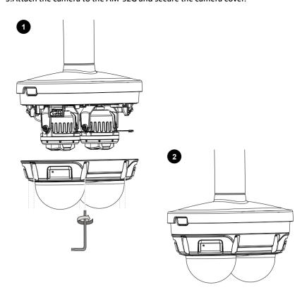
3. Install the camera, connect the IO cable, and adjust the waterproof plug and the position of the excess cable.
