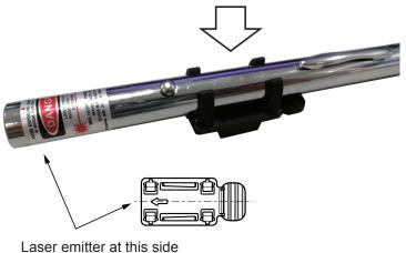
Select a laser pen with an approximate diameter of 12.5mm.
